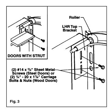
NOTE: Do not tighten fasteners for top brackets all the way until springs are installed and door is ready to be used. This way you will be able to make final adjustments if needed.
