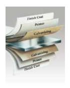
Steel skins are protected through a tough, layered coating system, including a hot-dipped galvanized layer, a protective metal oxide pretreatment and a baked-on primer and top coat.
