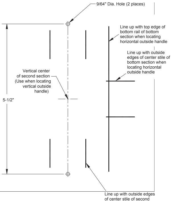
Line up with outside edges of center stile of second section when locating vertical outside handle
